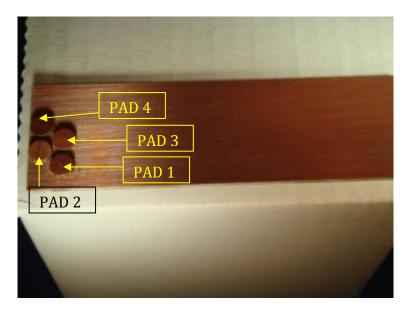
Superglue four pads to the PC board. Make sure they are not touching each other. You should have roughly 1/8 inch between the pads. Apply a small drop of superglue on the board and press the pad onto the board with the small dimple up. Use a small screwdriver to hold pressure on the pad until the glue dries (about 10 seconds).
