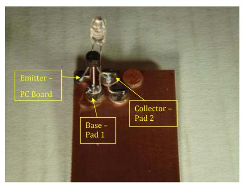
Solder the transistor to the board. With the flat part facing you the left lead (emitter) is soldered directly to the PC board. The center lead (base) is soldered to pad 1. The right lead (collector) is soldered to pad 2. Failure to install this part correctly will prevent the Joule Thief from working.
