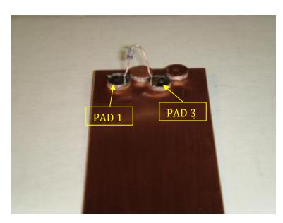
Solder the 1,000 ohm resistor onto pads 1 and 3. When soldering all components, place a 90-degree bend on the ends of the component where they touch the pad to allow better soldering. There is no polarity on a resistor.
