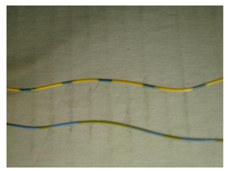
Take the two pieces of wire and **untwist** them if they are twisted. The toroid requires 12 inches of wire. You will wind the toroid with this pair of wires side by side.
