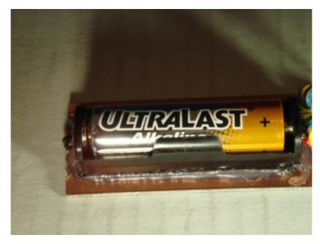
Solder the battery holder. Connect a short piece of wire from the positive terminal (the one without the spring) to pad 4. Solder the negative terminal (the one with the spring) directly to the PC board using a short piece of wire. Use hot glue or some other glue to secure the battery holder to the PC
