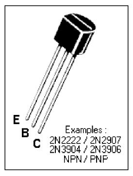
This is a diagram of the transistor showing the emitter, base and collector. Flat side forward, left to right.
