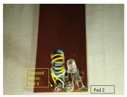
Solder the twisted wires on the toroid to pad 4. Solder one of the other toroid wires (doesn't matter which one) to pad 2.
