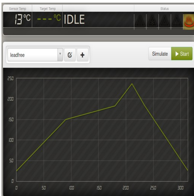
Illustration 1: picoReflow Temperature Profile for Lead-Free Solder (sample)
