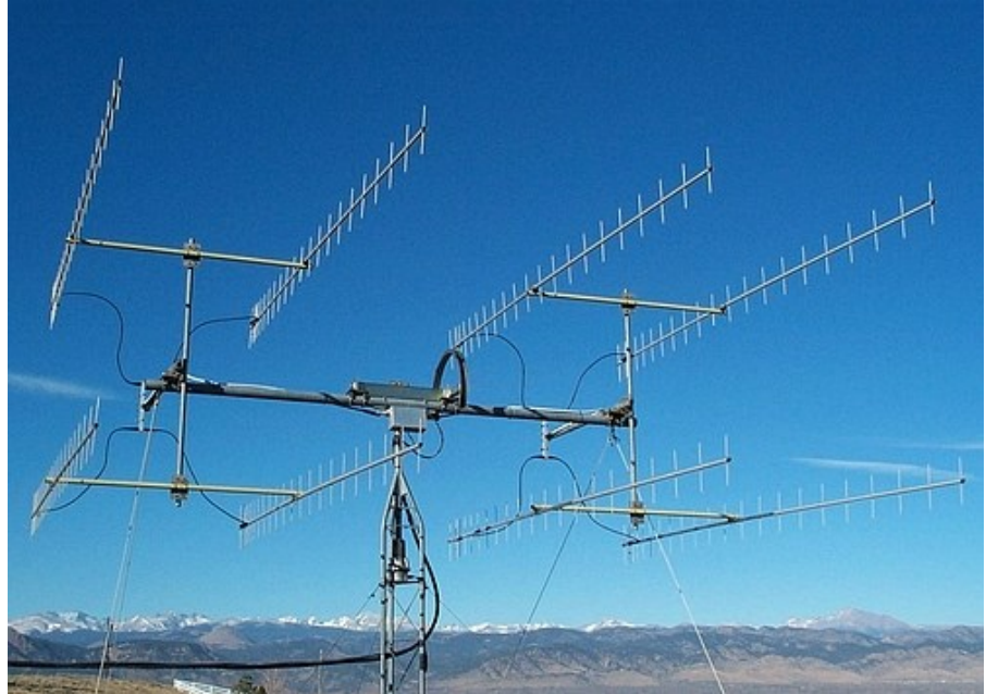
Typical EME array for 432 MHz. Maybe we made contact with this station!
