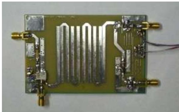
I was pleased that the transverter put out +15.25 dBm (or, approximately 32 mW). The TX side of the circuit took 187 milliamperes and the RX side of the circuit 120 milliamperes. The [1 db compression point](#) (or more formally, P1db) was at -2 dBm. So, at least for my transverter, I need to attenuate my radio to -2 dBm output drive in order to avoid saturating the circuit. Here, I used the following MMICs: A1=SGA3586Z, A2=MAR-6SM and A3=ERA-5SM.
